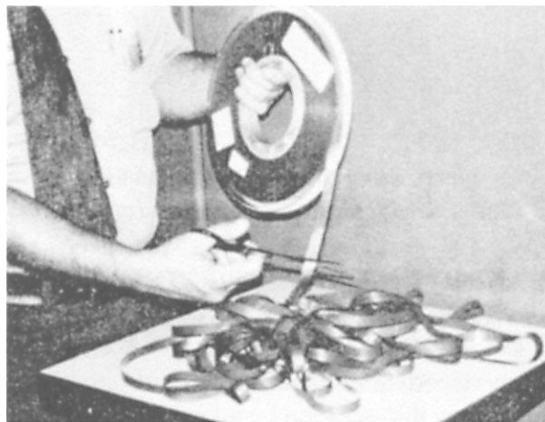
Figure 2-11.—A 100 feet of contaminated tape being removed from reel (stripping).
